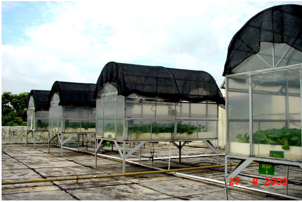
Plate 1. Development of the growth house prototype with CO 2 capability and minimal 'greenhouse effects' and fitted with CO 2 gas delivery and monitoring system
